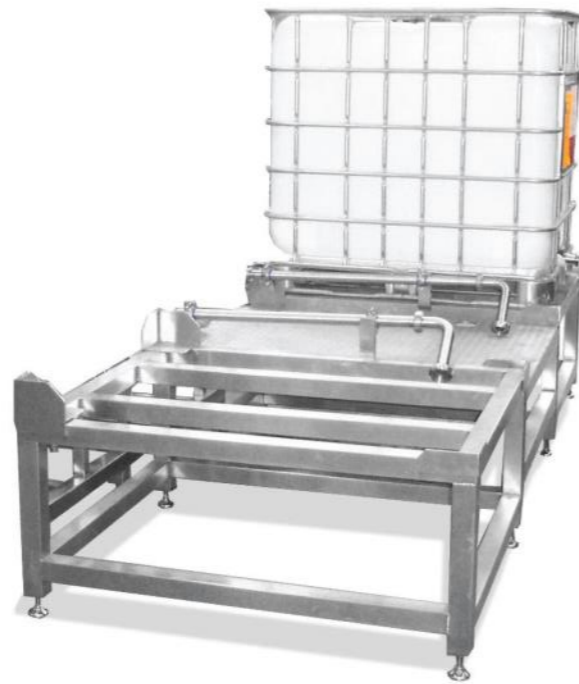
Typical 2 x IBC Internal Distribution Store
