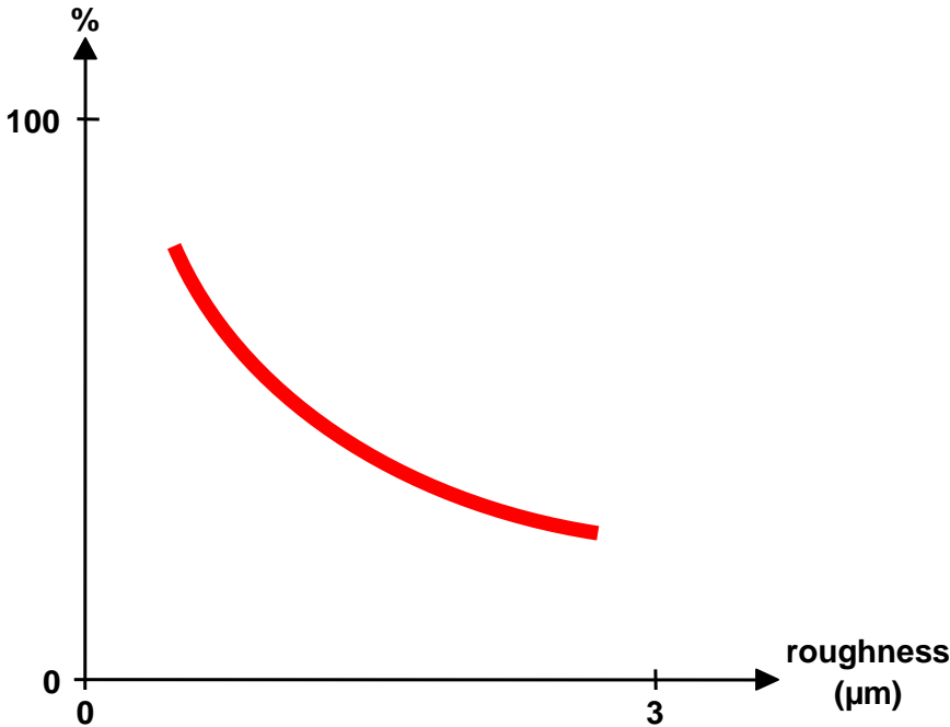
REDUCTION % OF MICRO-ORGANISMS AFTER A STANDARD CIP CYCLE (relative values)
